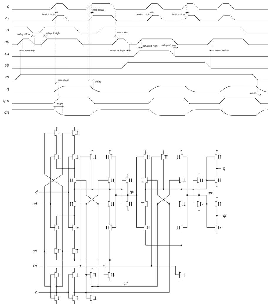
Figure 7: D flip-flop with scan inputs
