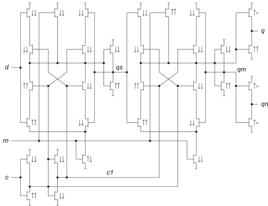
Figure 6: D flip-flop without scan inputs
