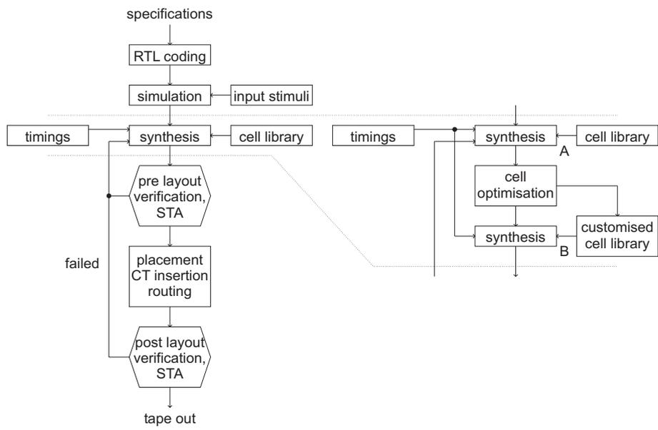
Figure 1: Digital ASIC design flow
