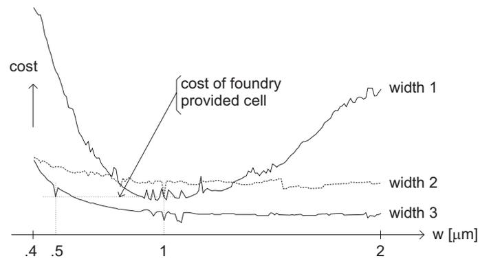
Figure 8: Cost function profiles for three transistor widths
