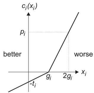
Figure 2: Measurement contribution function
